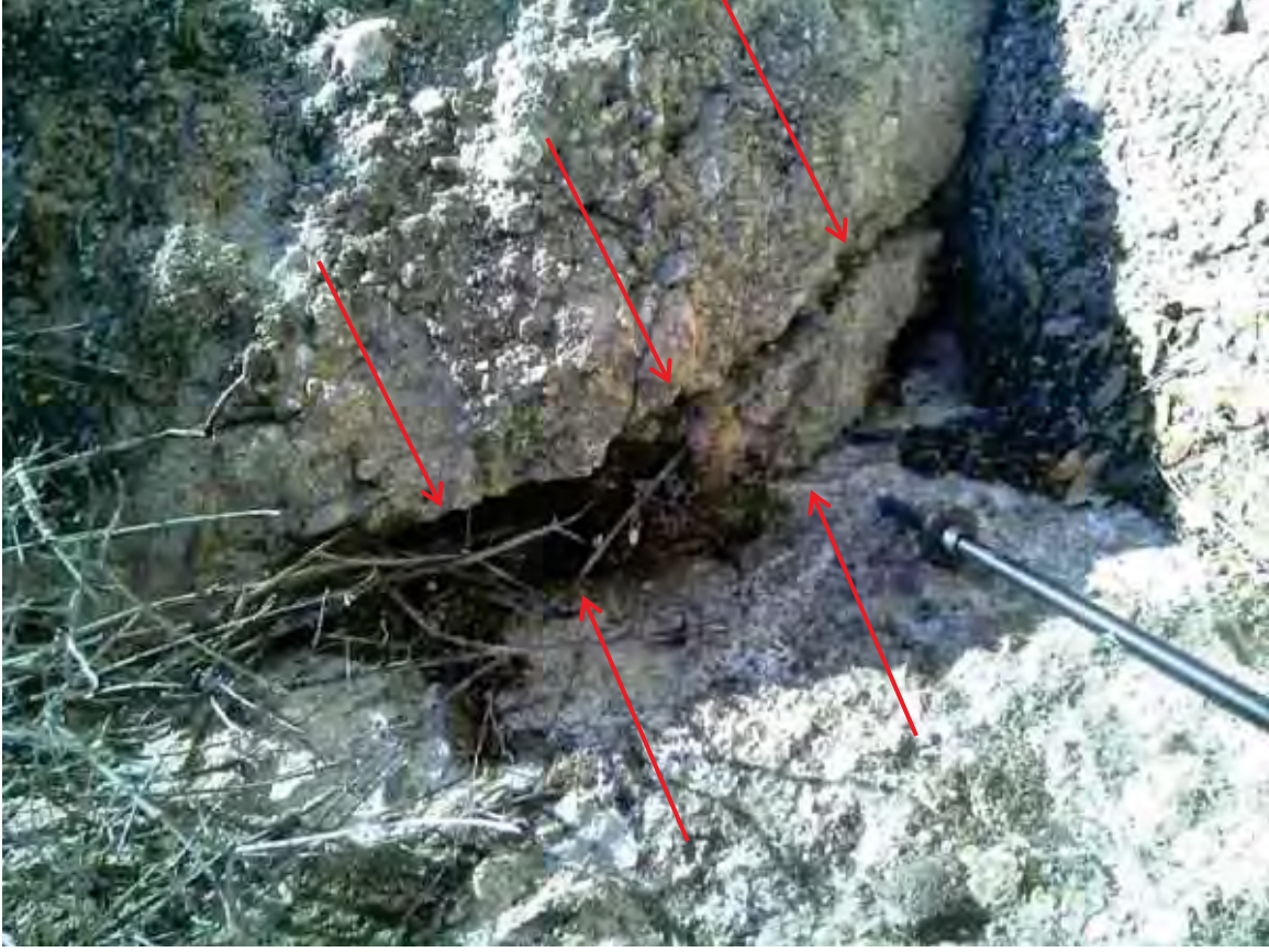
Photo No. 22 – Location 19: close-up of open fracture (hiking pole for scale).
