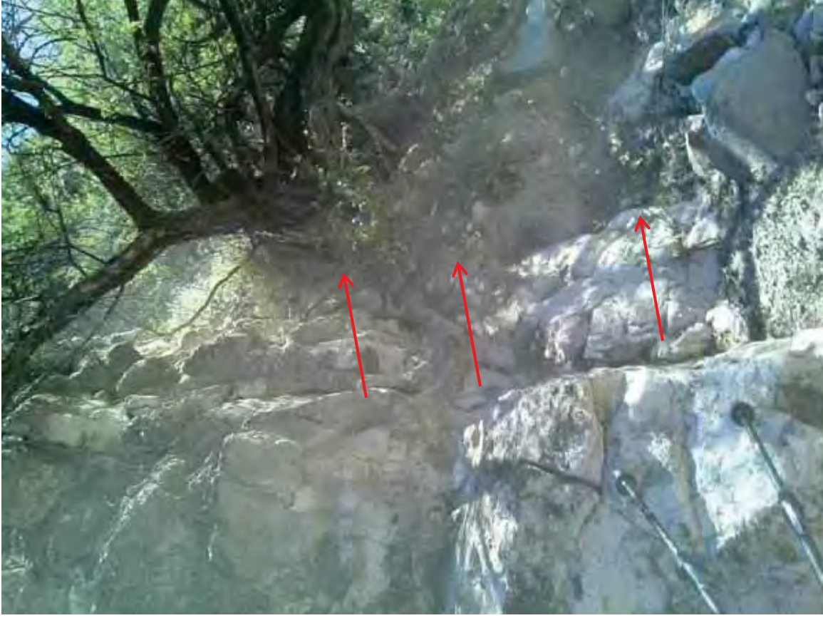
Photo No. 39 – Location 21: Partially-open vertical fracture in tuffaceous sandstone member of Big Dome Formation, adjacent to fault on right (hiking poles for scale).
