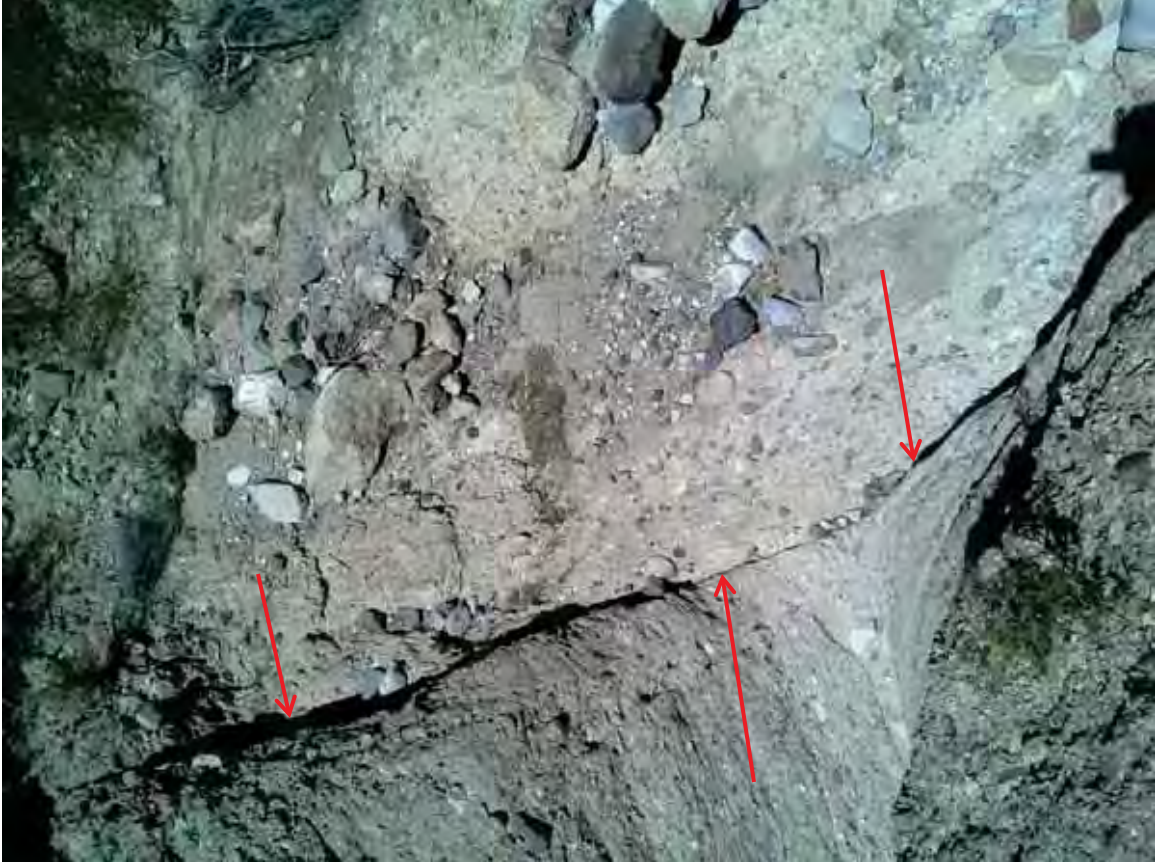
Photo No. 13 – Location 16: Looking down at partially closed to several inch aperture, sharp fault contact in Big Dome Formation crosses drainage; eroded by scour.
