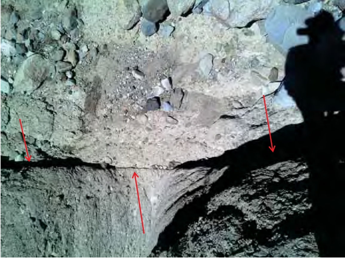
Photo No. 14 – Location 16: Looking down vertically at partially closed to several inch aperture, sharp fault contact in Big Dome Formation crosses drainage; eroded by scour.
