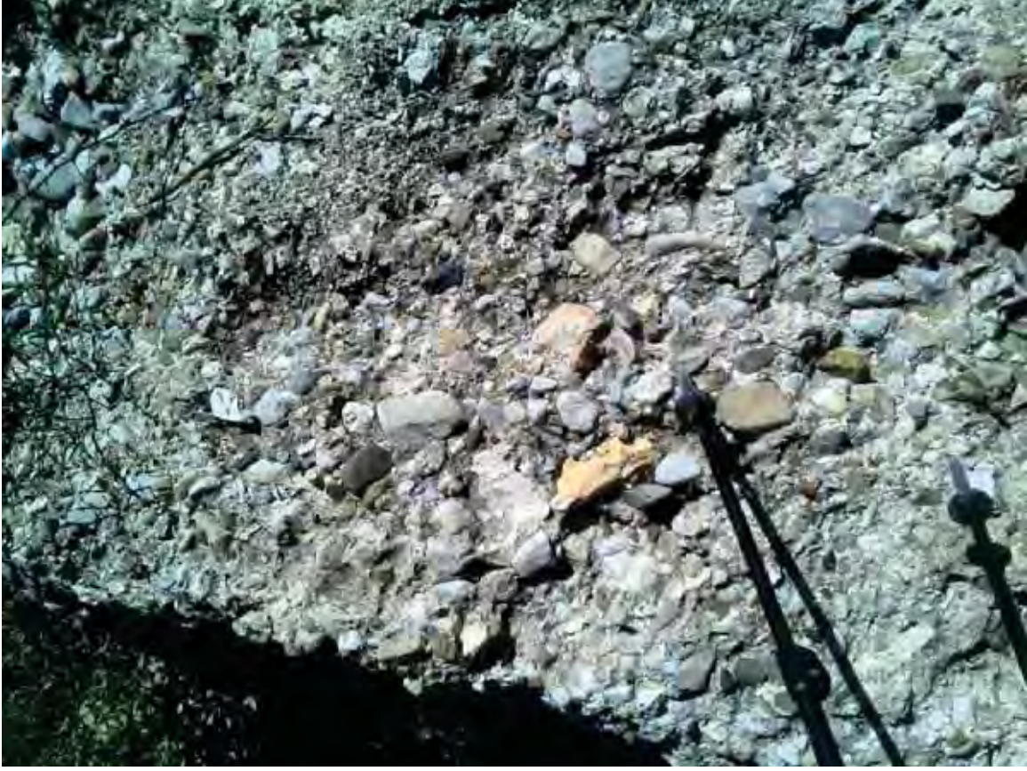
Photo No. 35 – Location 21: Typical conglomerate clasts in Big Dome Formation.
